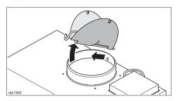
■ The non-return flap is not needed for the recirculation mode. Pull the non-return flap off the bracket from the vent connection.
